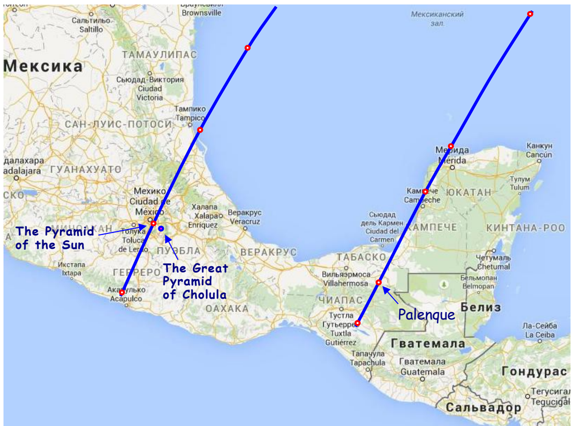
Fig. 10.10. Lines of equal azimuths (C) for the observation site ( 50.19111^\circ N, 36.28028^\circ E)
